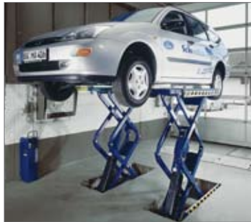
JUMBO LIFT I – extendable platforms
